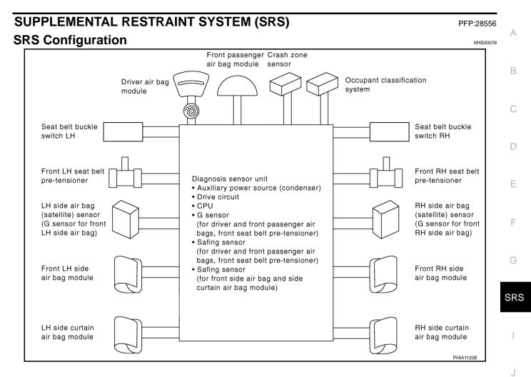
The air bag deploys if the diagnosis sensor unit activates while the ignition switch is in the ON or START position.
